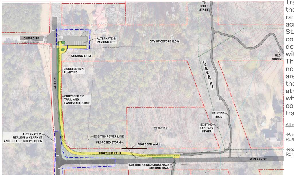
Trail begins at the existing raised crosswalk across W Clark St. The trail will continue west down W Clark St within R.O.W. The trail turns north at Hull St are runs north to the intersection at Oxford Rd, where it concludes with a trailhead.
